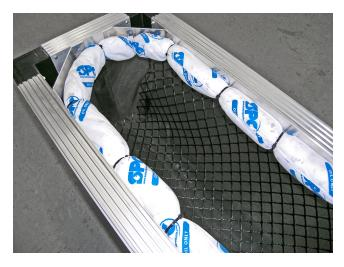
The oil boom kit can be added to any standard StormSack unit. During manufacture Fabco adds permanent mounts to the StormSack frame and then wraps a replaceable polypropylene oil-only absorbent boom around all internal surfaces.
